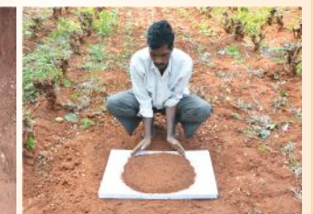
Mixing and spreading of soil sample
