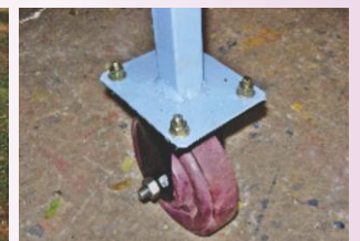
Swirling wheels for easy transportation of machine
