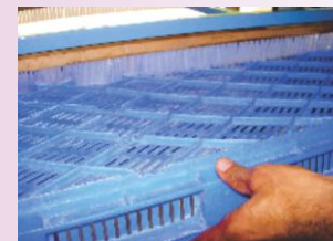
Brushes for rubbing of the trays for dirt removal
