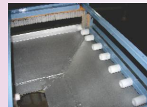
Nylon rollers for easy movement of the trays
