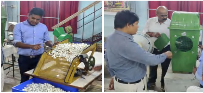
Manual cum motor operated table mounted deflossing machine and humidifier
